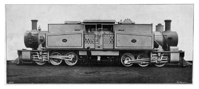
The Vulcan Foundry, Limited, of Newton-le-Willows, has recently built a powerful Fairlie type locomotive to the order of Messrs. Rendel and Robertson, Westminster, for the Mexican Railway. The engine is one of a batch of three constructed to haul trains weighing 300 tons up inclines of 1 in 25, combined with a five-chain curves and the gauge is 4ft. 8<sup>1</sup>/<sub>2</sub>in. The three engines each weigh 138 tons in working order.
